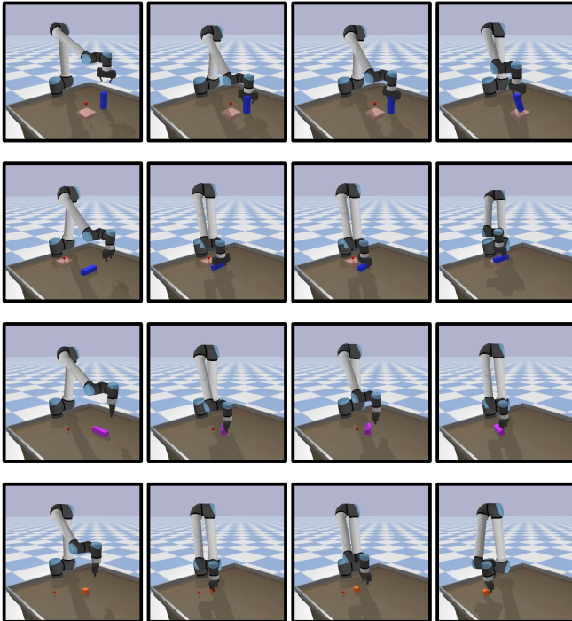
Fig. 6. Planning examples of our approach for Block Z, Block Y, Block X, and Cube objects (from top to bottom). The red dots show the goal position in each case. The top two rows belong to Task 2, and the bottom two rows show Task 1.
